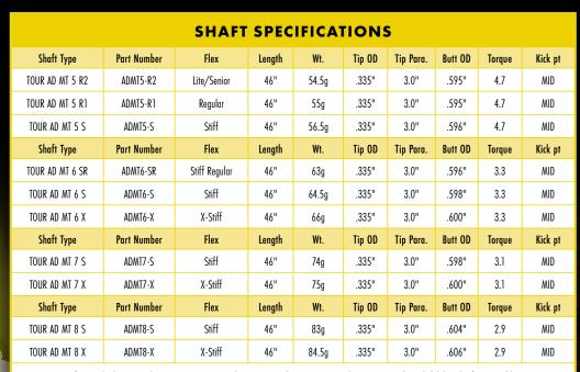
Tip Trimming for Standard Bore Heads: Driver: 0.0", #3 wood: .5", #5 Wood or greater 1.0", then Butt Cut to desired club length after assembly.
